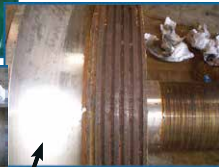
Rotating assembly showing worn and eroded seal rings and shaft sleeves
