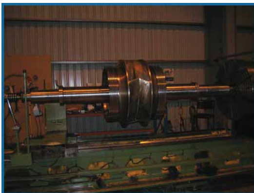
Refurbished assembly with new sealing rings and shaft sleeves
