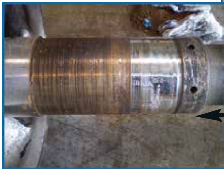
Rotating assembly showing worn and eroded seal rings and shaft sleeves
