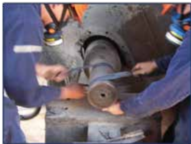
After building up the shaft with Belzona 1111, the former is removed, and the excess Belzona ground off
