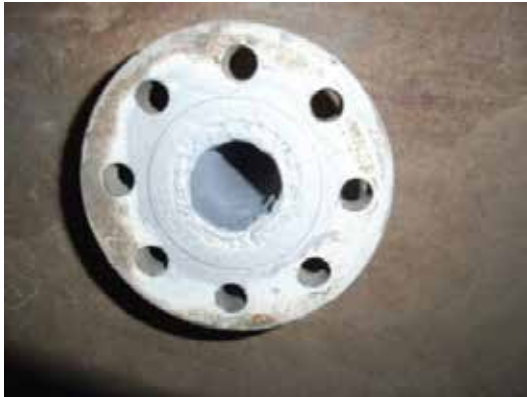
Blasting prior to application
