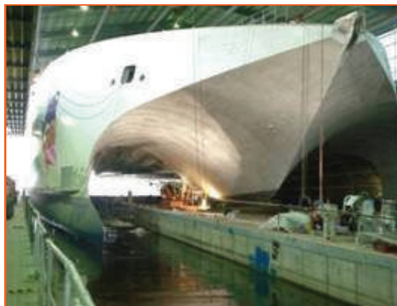
The vessel after blasting with Sponge-Jet
