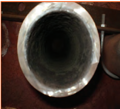
Typical coak, thickness 4mm, to be removed
